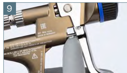
Grease visible part of air piston rod
